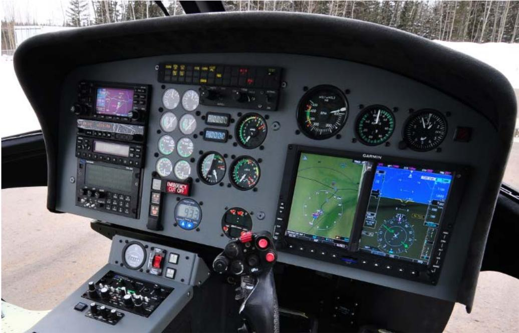
AS355N with Garmin G500H, GNS430W, GTS800, RA-4500 & Customer Specified Avionics Package
